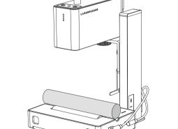
In [cylinder] mode, if the cylindrical object is frictionless, please wrap silicone bands on it.
